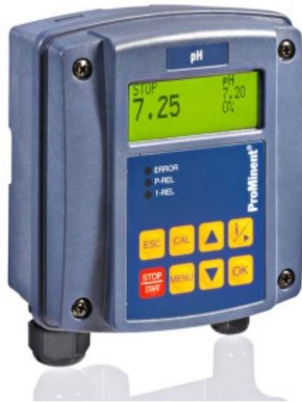
The DULCOMETER® Compact controller is a one-channel PID controller for the measured variables pH, ORP, chlorine and inductive conductivity. It can monodirectionally control the measured variable, monitor limit values and transmit the measured value via an mA output, e.g. to a PLC. The mA output can optionally also be configured as a controlled variable output. The controller has one pulse frequency output to control one metering pump. One output relay can optionally
